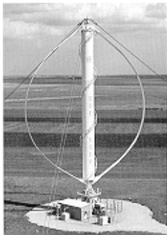
Fig. 4 Vertical-axis turbine (Darrieus design)
